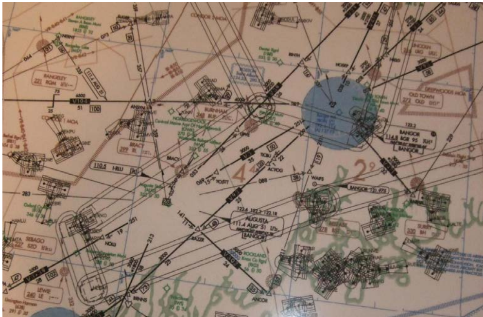
Figure 18 Example of privately developed Special Route that provides connectivity with Point-in-Space instrument approaches. Courtesy of LifeFlight of Maine.
