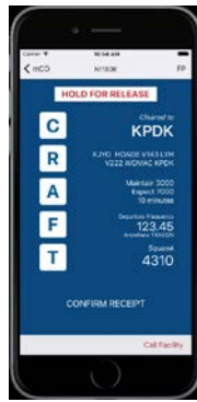
Figure 19 Screenshot from MITRE Prototype App for Electronic Transmission of Pre-Departure Clearances
